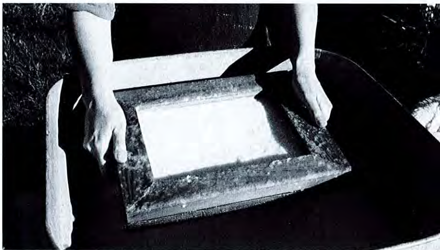
When you have a layer of pulp on the screen, raise the deckle and let the water drain.
